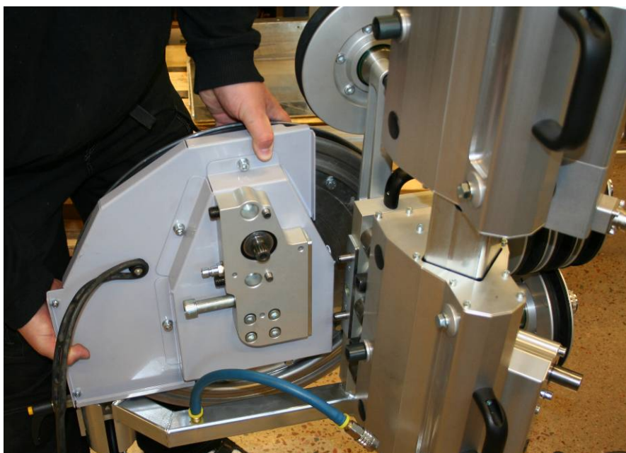
Fitting of main drive pulley assembly
