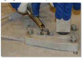
1:4 When the fork is completely turned in, turn the fork about 5 times counter-clockwise, to make sure the saw arm doesn't touch the concrete at the last cut if the concrete is uneven.
