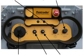
Movement of saw arm/ along the track/column Water ON/OFF HF-motor ON/OFF
